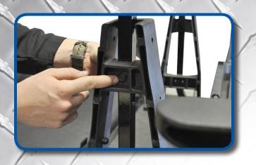
Now that your top is attached the rear struts can be secured. Using C-Clamps set rear struts to desired height. Using a 5/16" Drill bit, drill through struts using main mounting bracket holes as a guide. Attach with hardware from Pack#1 of your seat kit.
