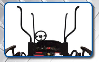
To attach the new struts to your G250/300 seat kit you will first need to insert them into the main brackets as shown. DO NOT drill any holes in strut until Step 7.
