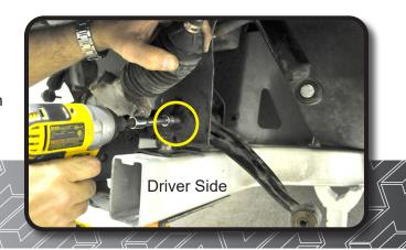
Note: Grease all fitting before installing lift on Cart. 1 each on the upper A-Arms and 2 on each on lower A-Arms
