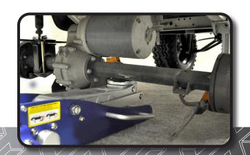
NOTE: After the first hour of drive time, re-check all lift kit components and alignment. Regrease the fittings, check the alignment and ensure all lift kit hardware is secured for safety after 50 hours of recurring use.
