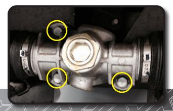
Using spring plate retained from Step 8. Attach your new main suspension assembly. Use the supplied M10x45mm hex bolts to secure to cart.
