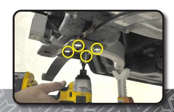
Using a 1/2" Socket remove 3 bolts securing rack and pinion. Retain hardware.
