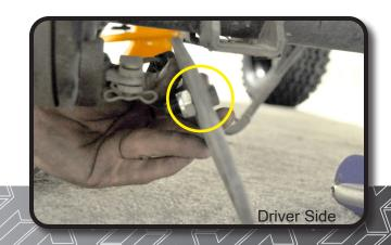
Route U-Bolt through Shock mounting plate around axle and through factory lower bracket making sure alignment bolt attached in step 27 fits properly in axle. Using a 17mm socket tighten U-Bolt evenly to ensure proper alignment.
