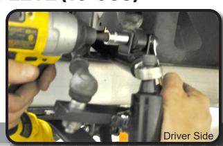
Reattach hub using hardware retained from Step 4 and tighten.
