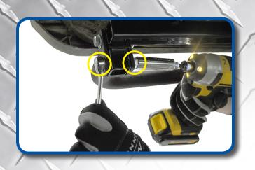
Using the 10mm x 55mm hardware provided attach step to bracket using 17mm socket and wrench. Once all 4-bolts are in place then tighten.
